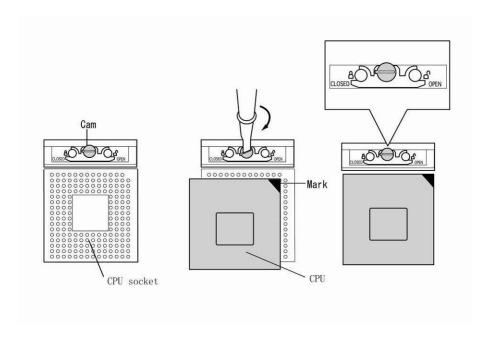
Figure 4-39 Installing the CPU
